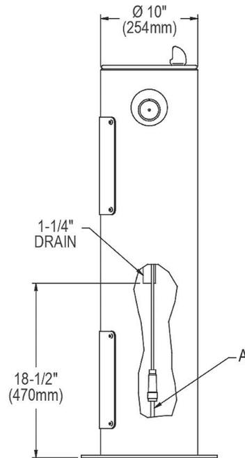
A = 3/8" O.D. UNPLATED COPPER TUBE CONNECT
